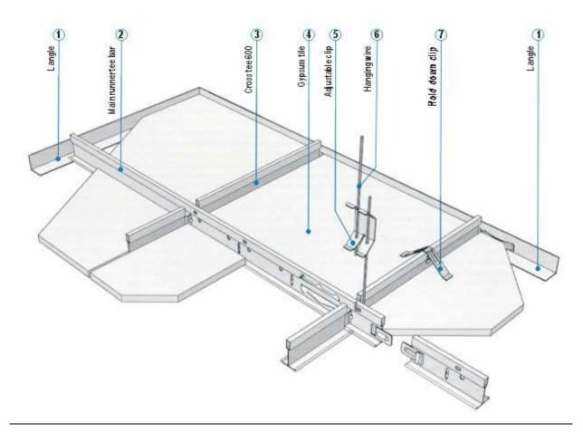
The system is a lay in system which uses acrylic aluminium laminated gypsum panels of size 600x600mm laid on exposed suspended metal ceiling tee bar grid system. Main components and material specifications:
